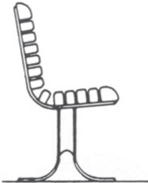
Portable base: 3/8" x 2 1/2" formed steel continuous welded to 3/8" x 2 1/2" stiffener plate between legs.
