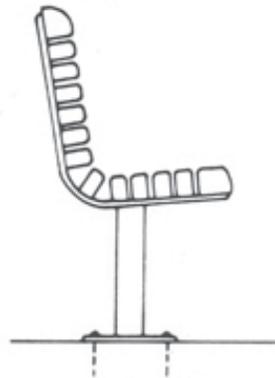
Surface mount: 2 1/2" squared steel tube welded to 3/8" x 4" x 9" base plate with holes for two 1/2" anchor bolts 7" apart.
