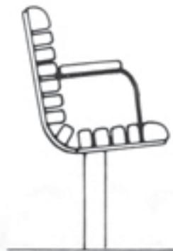
Armrest available for most benches. 3/16" x 2" formed steel plate is welded to the bench frame and supports 2" x 3" wood arm.
